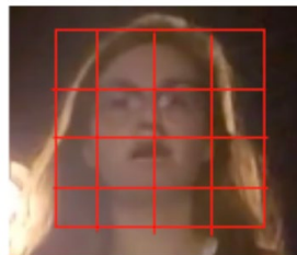
Figure 2. “Area-of-Interest”. As seen in Figure 2, MTCNN neural network is detecting the face of a human in each frame, the box area of face detection is then matched with the tiles of the frame to constitute the “Area-of-Interest”. (Photo credit: https://www.kaggle.com/competitions/Deepfake-detection-challenge/data )
