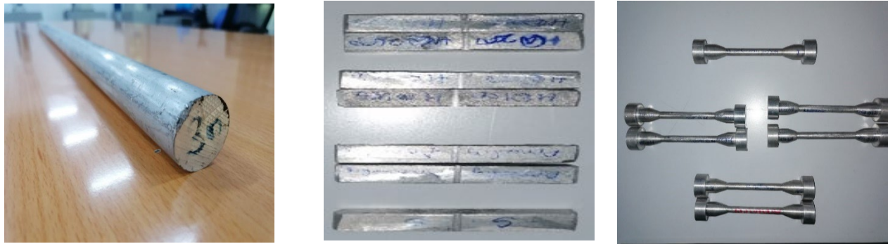
Figure 4. Show Aluminum 6061 alloy bar and its machined specimens
