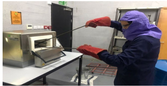
Figure 6. Placing of specimen in furnace
