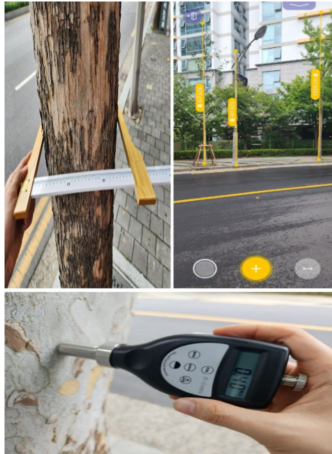
Figure 3a, 3b, and 3c. Photographs of field measurements for the variables using a specialized vernier caliper for measuring trunk DBH, an AR ruler for measuring tree height, and a wood densitometer for measuring tree density.
