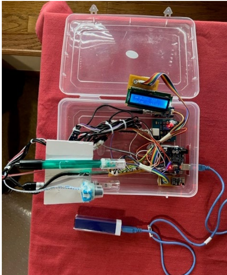
Figure 1. Picture of assembled Arduino with 5V power supply
