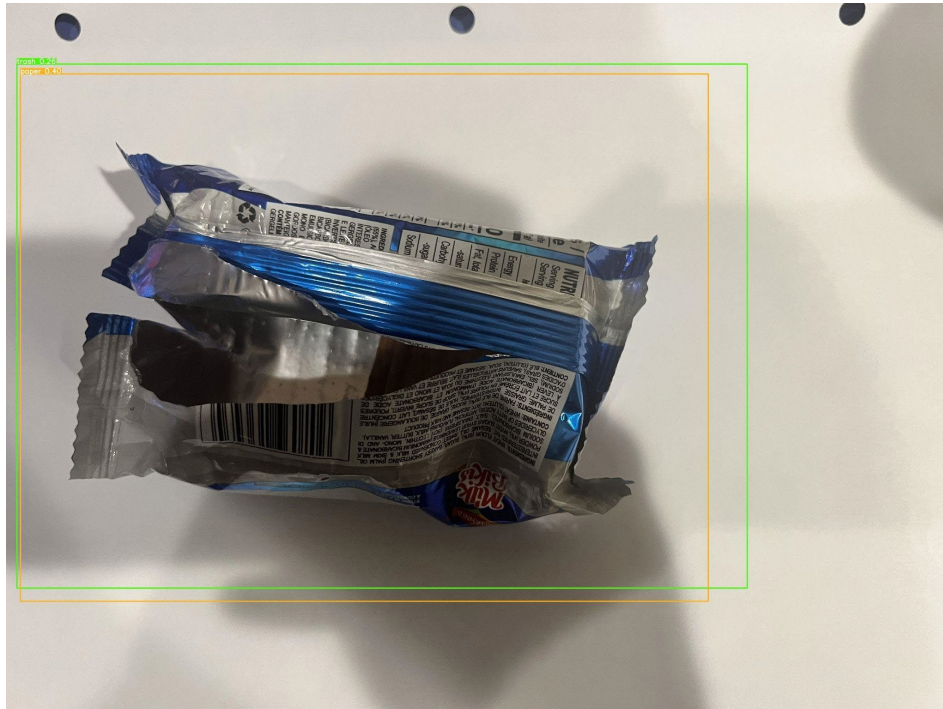
Figure 8. A piece of trash is classified as paper and trash simultaneously. The piece of trash shown here is an empty wrapper for some Indian biscuits, which the model has never seen before.
