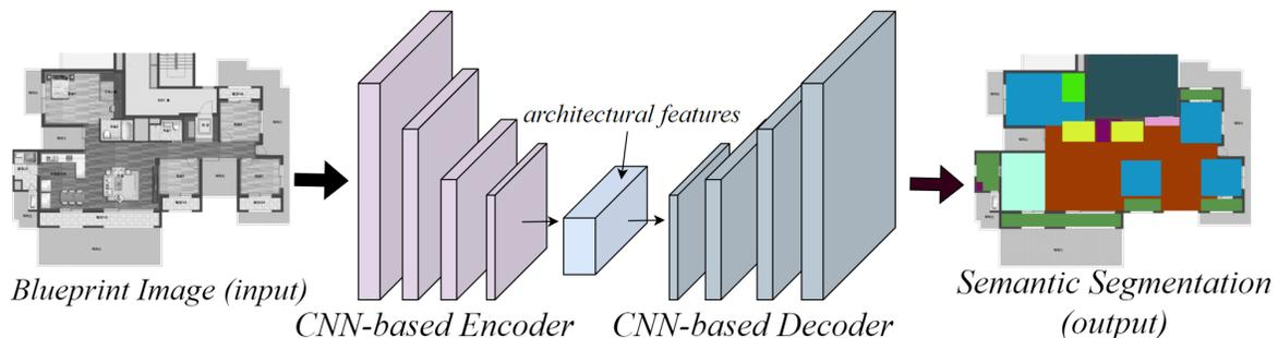
**Figure 3.** Diagram of the proposed blueprint segmentation system
