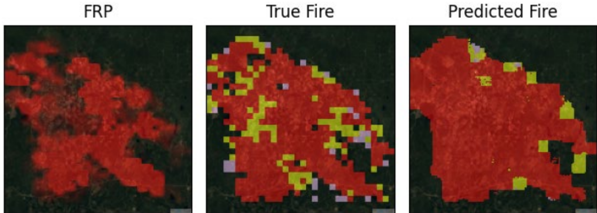
Figure 4. U-Net qualitative result for 2023 Canada Fox Creek wildfire. Predicted accuracy around the edges of fire regions is low. Segmentation class colors are 0 - no color, 7 - purple, 8 - yellow, and 9 - red.
