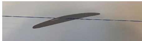
Figure 1. Example of top-down view of unstable disk due to a large distance between holes. The disk does not stay perpendicular to the line and does not spin effectively.
