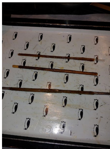
Figure 7. Bacterial cellulose straws applied with different oils: linseed and tung oil
