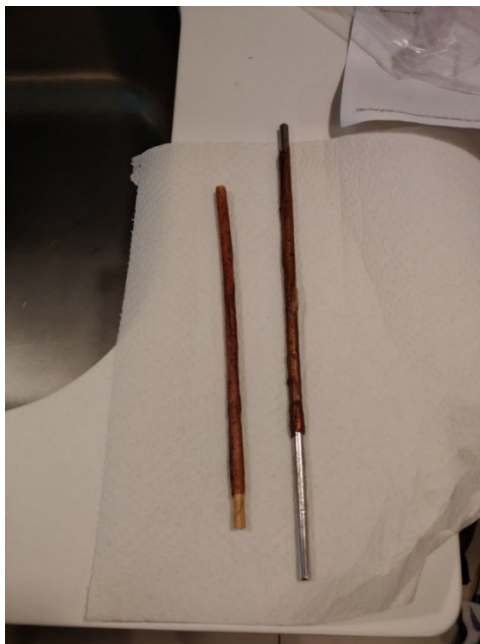
Figure 8. Bacterial cellulose straws are attached to the paper and metal straw, making paper and metal straws an unsuccessful molding device
