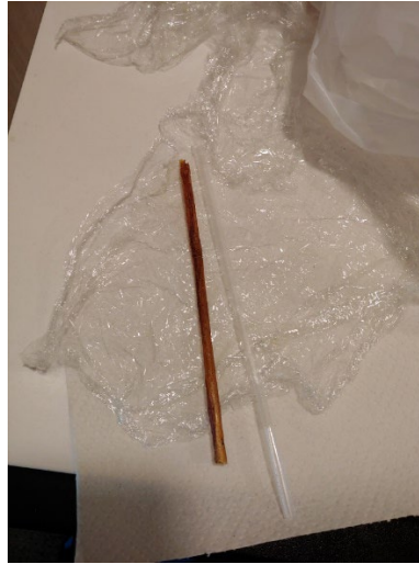
Figure 6. Bacterial-cellulose straw molded from a plastic straw structure (final drying process)
