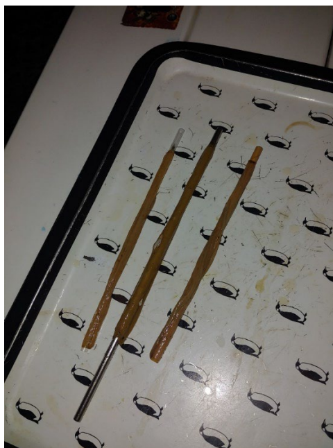
Figure 5. Bacterial cellulose being molded on different types of straws: paper, plastic, and metal
