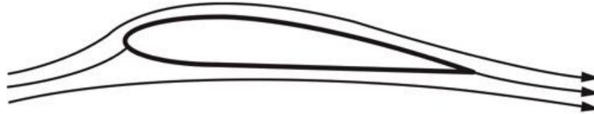
Figure 15. Streamline pattern at a low angle of attack. Figure taken from (McLean 2013).
