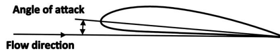
Figure 3. The geometry of an airfoil showing the angle of attack between the chord line and flow direction (Mclean, 2014).
