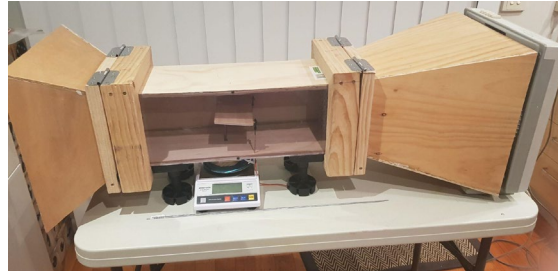
Figure 6. Final constructed wind tunnel with digital scales and box fan.
