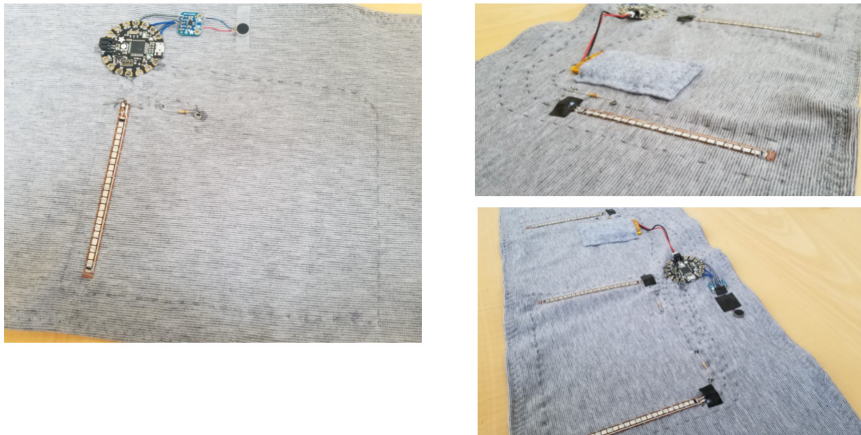
Fig. 12. Using conductive thread to connect electrical paths.
