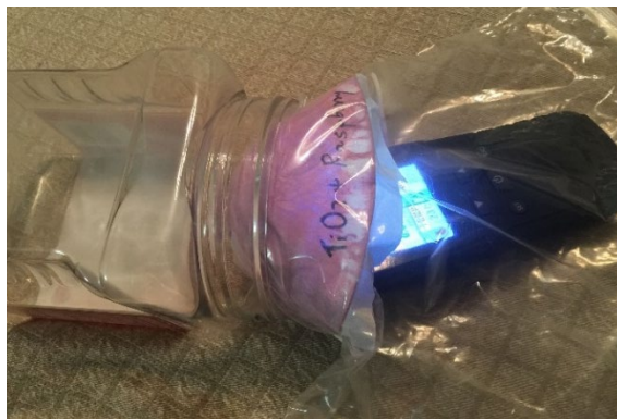
Figure 3. Horizontal view of experimental setup with smoke chamber and testing chamber
