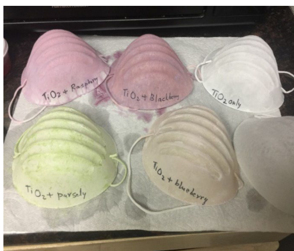
Figure 2. Air-dried Dye-Sensitized TiO 2 filters
