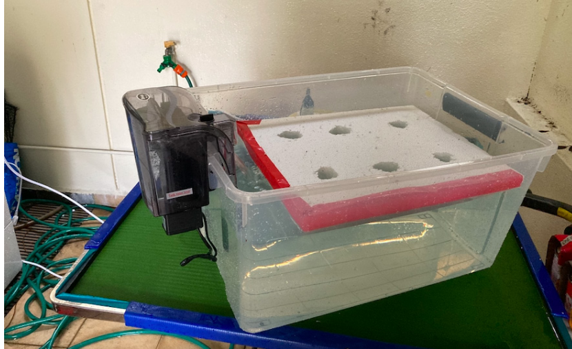
Figure 4. The Raft System fully assembled during building process
