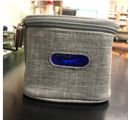
Figure 4. Front view of Vemingo device. Figure 5. Side view of Vemingo device. The right is the side view of the device when it is on. The small window shows when the device is in use, as the blue UV-C light can be seen on.
